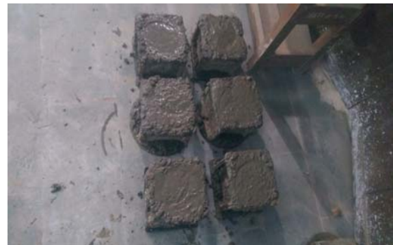
Figure 5: Mold filled with proper mix design material
